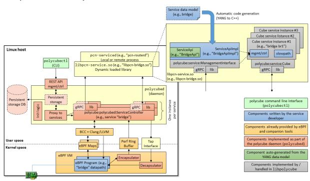
The architecture includes four main components: *polycubed*: a service-agnostic daemon to control the polycube service, a set of *polycube services*, which actually implement the network functions, *polycubectl*, a service-agnostic CLI that allows to interact with polycube and all the available services, and *libpolycube*, a library that keeps some common code to be reused across multiple network functions.
